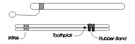
2. Put the 2 sticks on top of each other with the wires touching. Wrap a rubber band tightly around the other end.
