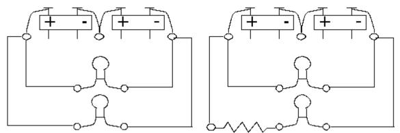
3. With the resistor in the circuit, observe and record what changes have occurred in the two lights.
