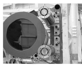
Earlier this year the team assembled a prototype double-barreled x-ray telescope consisting of two mirror assemblies with three shells each. It passed laboratory tests with flying colors, but that wasn't enough. An x-ray telescope on the ground is like an optical telescope with the lens cap on. "Cosmic x-rays don't reach Earth's surface," explains Ramsey, "because our atmosphere is opaque to this high energy radiation." It was time to go to space -- or as near to it as they could get.
