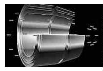
"Focusing hard x-rays is difficult, because they are absorbed by conventional lenses and mirrors," explains Ramsey. "The only way to reflect a hard x-ray photon is to bounce it from a mirror at grazing incidence -- that is, at a very shallow angle." It's a little like skipping stones across a stream. The rock (or x-ray photon, as the case may be) will skip only if it glances off the surface at a small angle. "The reflection angles for x-ray mirrors are just a few
