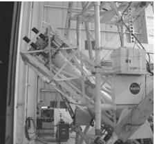
we've done so far is just a proof of concept." In two to three years Ramsey's team hopes to fly a balloon laden with 240 x-ray mirror shells. "That telescope will be sensitive to hard x-ray photons up to 75 keV, and it will produce images with 15 arcsecond resolution." (The May 2001 experiment flew 6 mirror shells, and was sensitive to 50 keV photons at 45 arcsecond resolution.)
